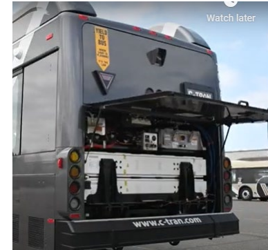
Probable Cause: Coolant leak in rear ESS
